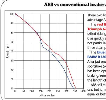
These two lines demonstrate the advantage ABS can give you. The **red line** shows a 2008 Triumph 675 Daytona with a skilled rider going from 100mph to 0 as quickly as he can, on a dry but not particularly grippy road. After three attempts his best is 356 feet. The **blue line** shows a 2008 BMW R1200GS fitted with ABS. After just one run it beats the little sportsbike (whose centre of gravity
